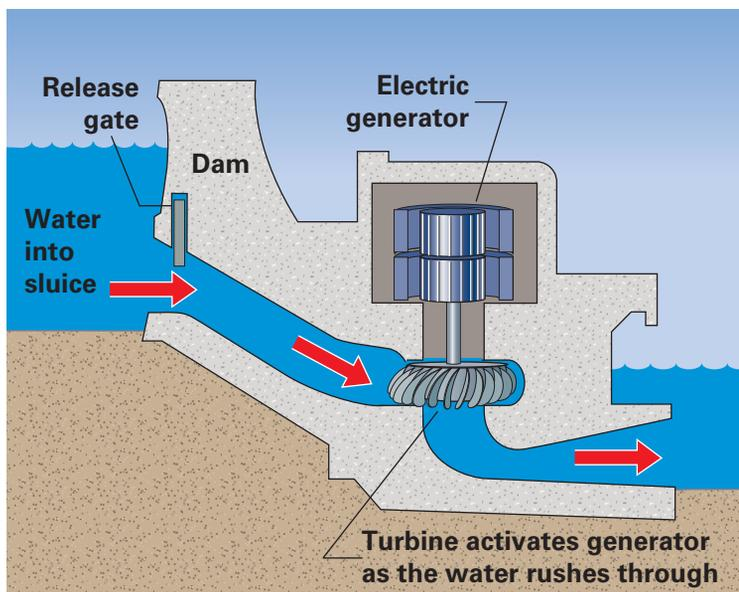
**Going with the Flow** Water flowing through the dam spins a turbine connected to a generator. *What is another term for water power?*
